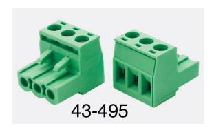
Two-part terminal-strip connectors. The free part has screw terminals for the incoming cable and plugs into the fixed part built into the equipment. Most manufacturers using these connectors supply both parts of the connector with the equipment, but the free part is also offered separately for pre-wiring, testing or maintenance. Each connector has three pins and carries one audio circuit.
